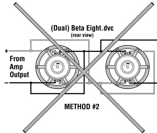
**IMPORTANT:** When connecting two Beta Eight.dvc subwoofers together, use Method #1 to create a net 4-ohm impedance. NEVER USE METHOD #2, since most amplifiers cannot fully control driver movement in this configuration.
